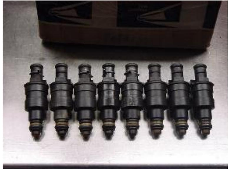
Next, each injector is engraved with a serial number. This permanent number allows each injector to be tracked through the servicing process and the data collected for each injector can be referred to weeks, months, or even years later.
