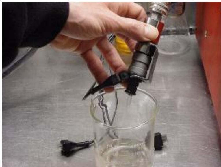
The injectors are then flow tested again in both static and dynamic modes. This data is recorded and compared to the initial flow data from before the injectors were cleaned.
