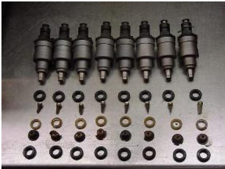
The first electrical test is to check each injector's ohm resistance. This tests the injector's coil windings for shorts or opens in the windings. The readings are noted on the injector service data sheet.
