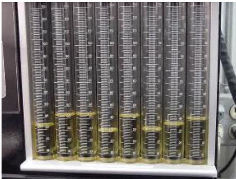
Now the injectors are flow tested again both statically and dynamically until one or more of the injectors reaches 100ml in flow.
