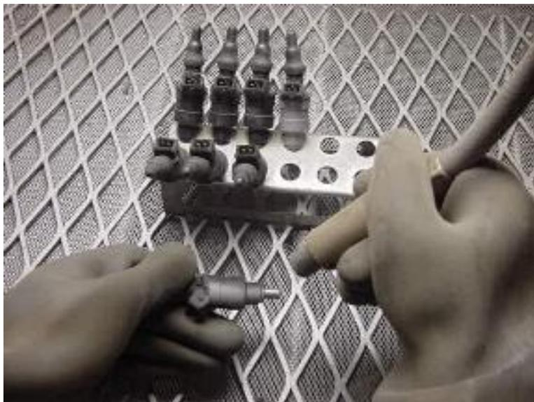
Next, the inlet screen is removed from each injector and the inlet of the injector is inspected for rust or corrosion.
