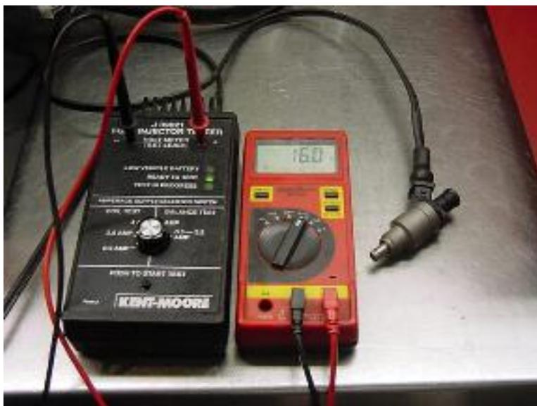
The second electrical test is a coil load test. This test checks the condition of the coil windings while in a "powered up" condition. The readings are noted and each injector is compared to the others for differences between the set of injectors.
