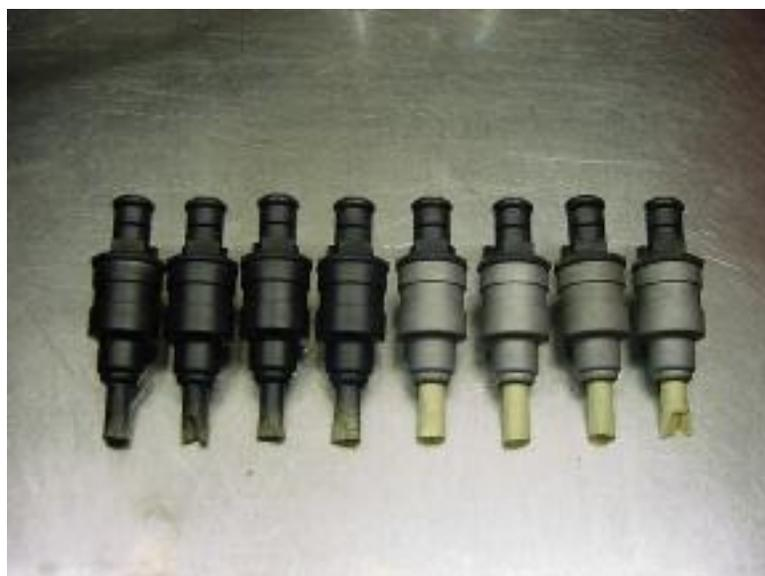
The injectors are now ready to reassemble with new o-rings, inlet screens and pintle caps (if applicable).
