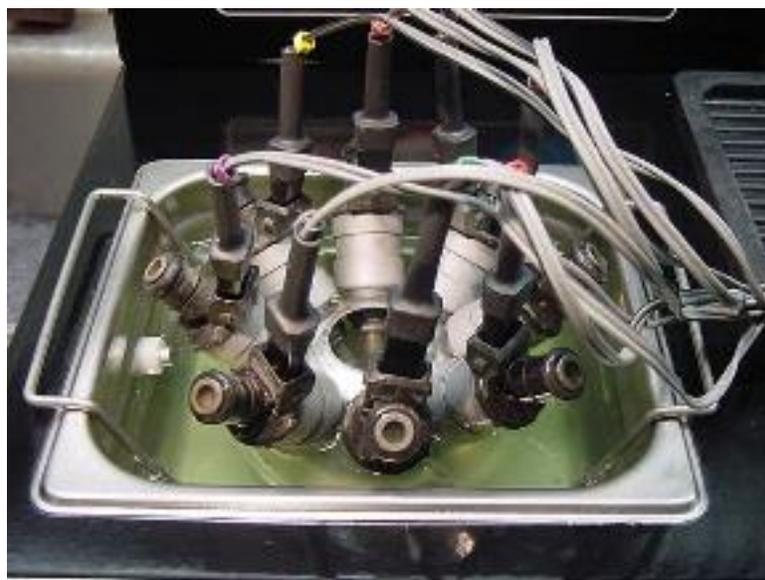
After the ultra-sonic cleaning process is finished, each injector is backflushed to remove the cleaning solution along with any debris that remains inside the injector.
