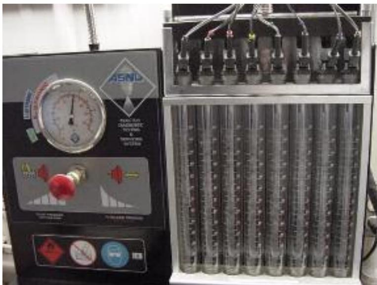
The next test is a visual test of the injectors while being flowed under pressure. The injector spray patterns are checked for uniformity. Any injector that has a "stringy" or abnormal pattern is noted.
