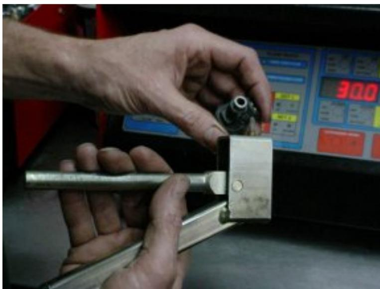
The last step in disassembly involves removing the remaining o-rings, pintle caps and spacers. The injectors are now ready for servicing.
